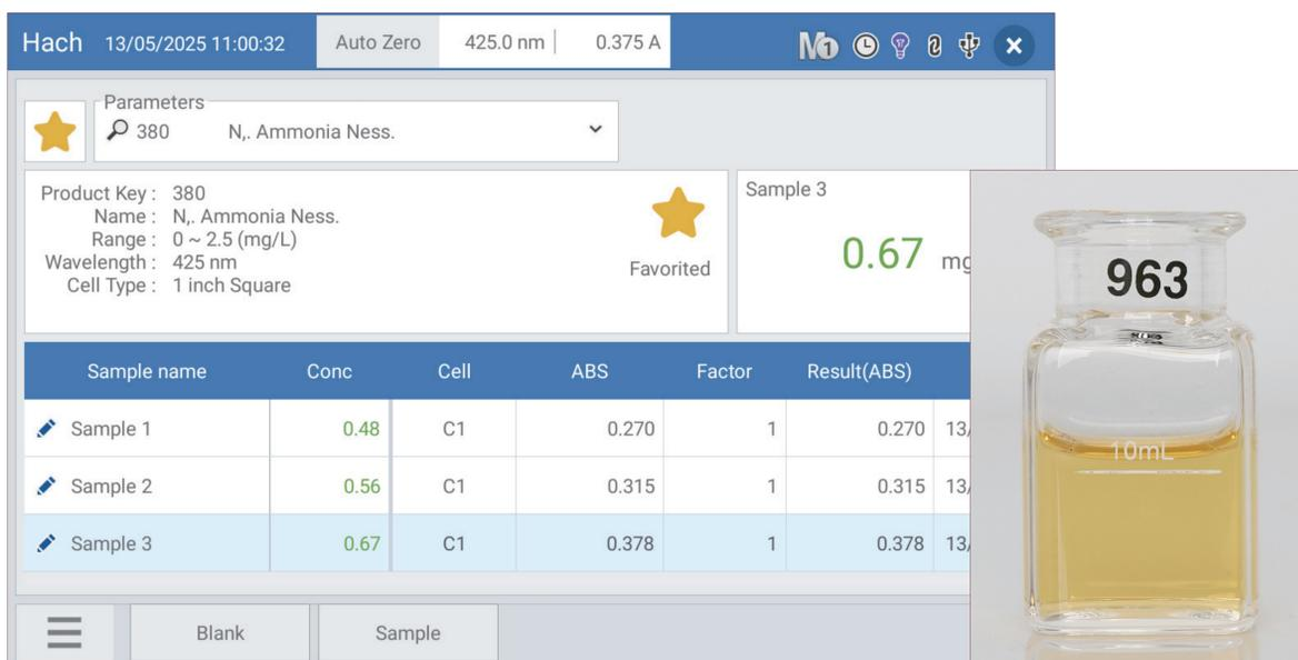
**[Figure 3]** QX [Sample] button and 1-inch cuvette (Sample)
