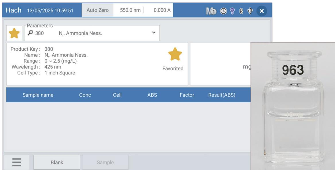
**[Figure 2]** QX [Blank] button and 1-inch cuvette (Blank)
