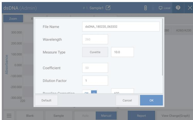
Fig. 2.12 [Change Measurement Type and Optical Path Length]
