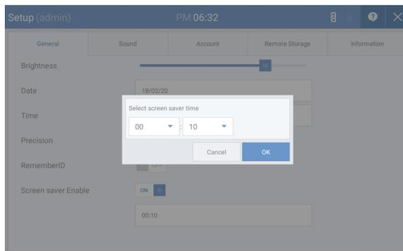
Fig. 2.6 [Screensaver Activation (Standby Mode) Time Setting]
